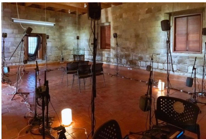
Figure 3: 16-channel loudspeaker setup at the MUSEUM [AUTHOR].
