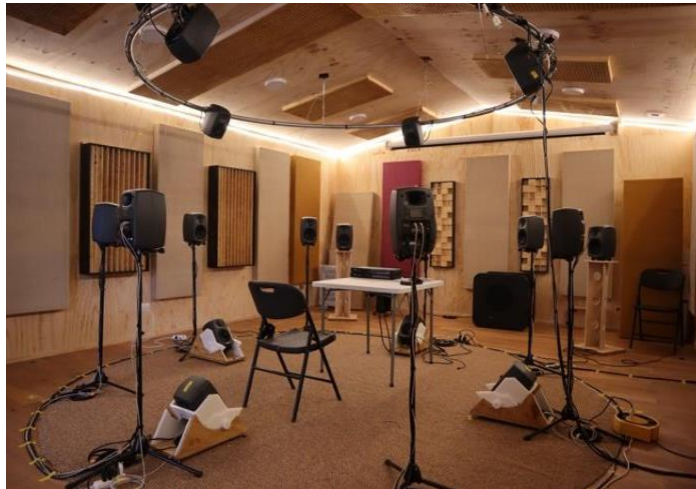
Figure 2: 12-channel loudspeaker setup in acoustically controlled environment used for the first part of the test. [AUTHOR].
